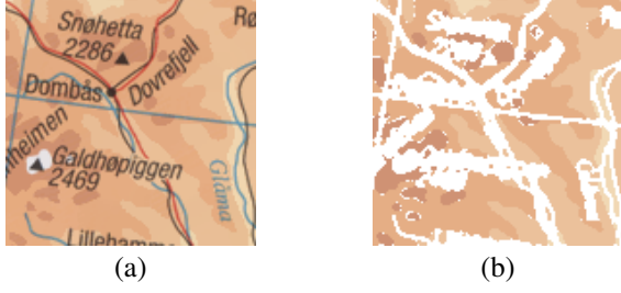
Figure 3: The map image. (a) After MEAN SHIFT filtering (spatial resolution h_s = 7 , color resolution h_r = 2 ). (b) The identified altitude layers - a map image that contains 4 colors to denote the elevation layers plus white to denote unclassified pixels.
