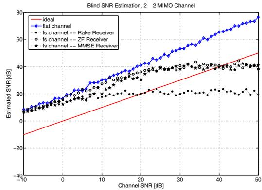
Figure 5: Estimated SNR vs. SNR for ST-Rake, TD-ZF and TD-MMSE, blind method used
