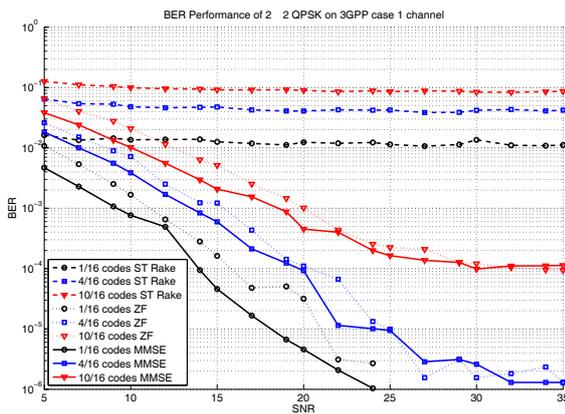
Figure 4: BER vs. SNR for ST-Rake, TD-ZF and TD-MMSE, QPSK used
