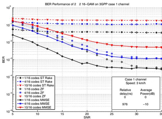
Figure 3: BER vs. SNR for ST-Rake, TD-ZF and TD-MMSE, 16 QAM used
