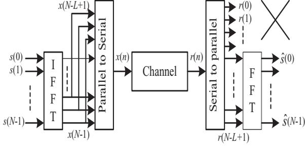
Figure 1: A basic baseband OFDM system, transmitting subsequent blocks of  $N$  complex data.
