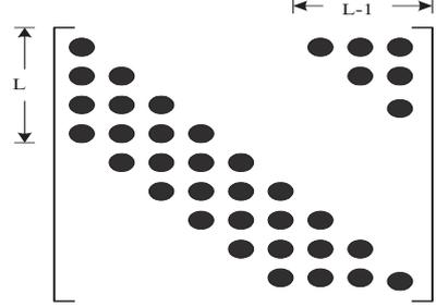
Figure 2: Diagonal structure of the time-domain CCM  $\mathbf{H}$ .
