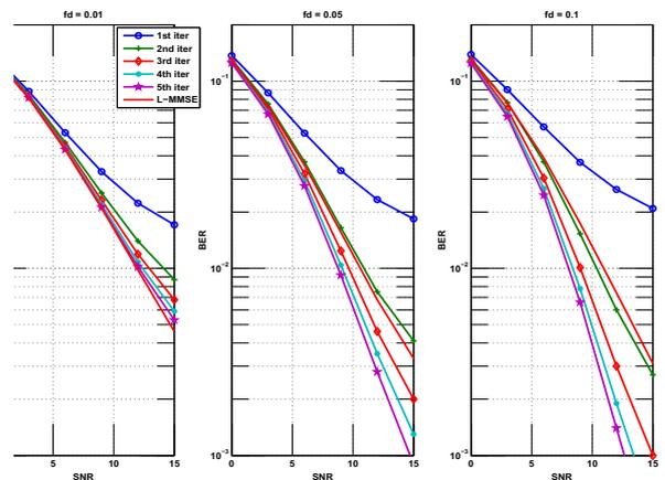
Figure 3: Comparison of BER performance of MMSE-iterative algorithm with the L-MMSE equalizer up to five iterations and at different DS.
