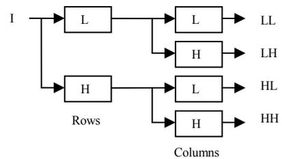
Figure 1. Illustration of discrete wavelet frame decomposition with lowpass (L) and highpass (H) filters. The input image is decomposed into four subbands.
