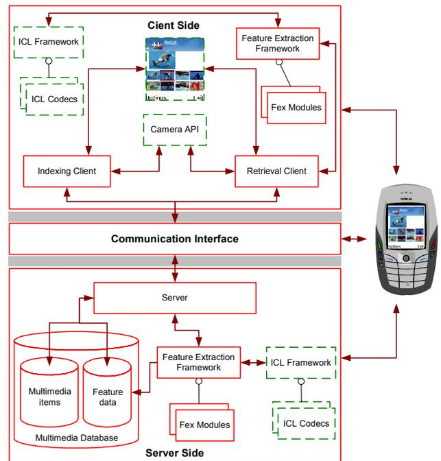
Figure 2: The proposed CBMIR framework for Symbian-based mobile platforms
