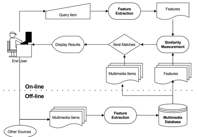
Figure 1: Overall content-based multimedia indexing and retrieval layout
