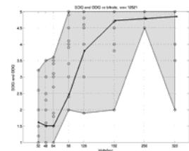
Figure 5: ODG (bold line), maximum SDG and minimum SDG (thin lines) vs bitrate for audio file 12521
