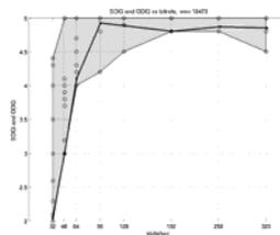
Figure 4: ODG (bold line), maximum SDG and minimum SDG (thin lines) vs bitrate for audio file 12473
