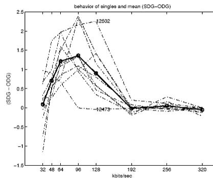
Figure 3: behavior of single and mean difference between ODG and average SDG
