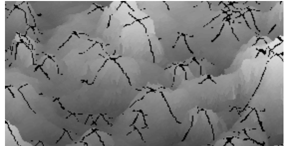
Figure 4: Detection of the clods for a portion of a seedbed’s surface
