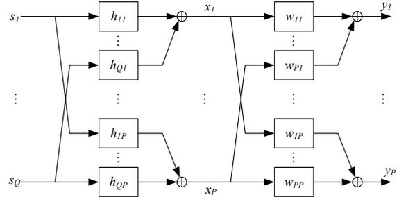
Figure 1: Linear MIMO model for BSS
