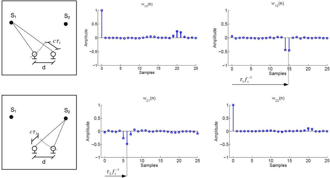
Figure 2: Sources configuration and corresponding de-mixing filters.
