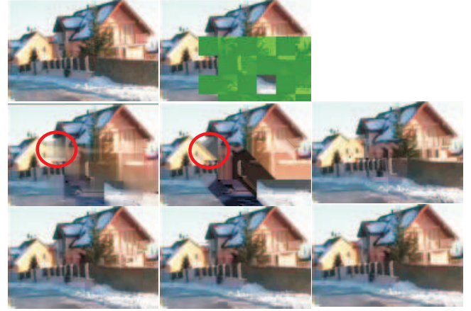
Figure 2: Screenshots of a part of an I frame in the "panorama" sequence (left to right): compressed original (Y-PSNR= 35.86dB), error pattern (Y-PSNR= 10.45dB), weighted averaging (Y-PSNR= 18.09dB), directional interpolation (Y-PSNR= 16.57dB), "copy-paste" (Y-PSNR= 22.76dB), boundary matching (Y-PSNR= 26.27dB), 8 \times 8 block matching (Y-PSNR= 30.27dB), 2 \times 2 block matching (Y-PSNR= 30.74dB).
