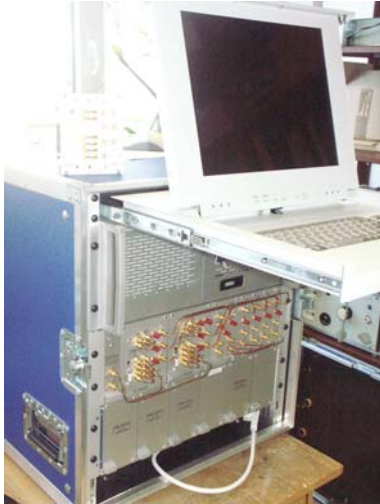
Figure 5 - Real-time UWB MIMO channel sounder design
