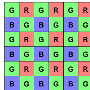
Figure 1: Bayer pattern used in the paper.
