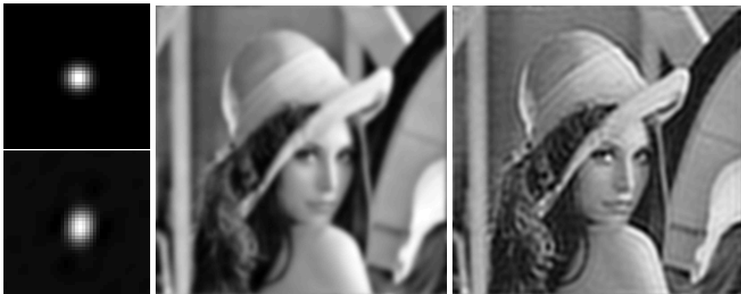
Figure 3: Gaussian PSF with small support. Images (left to right) of the true PSF that was used to generate the degraded image (top), the estimated PSF (bottom), the observed image and the estimated image.
