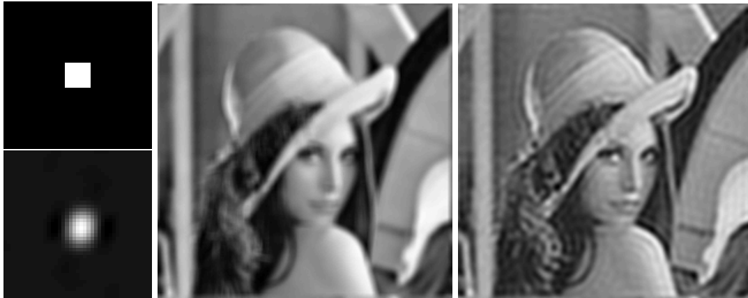
Figure 4: Square-shaped PSF. Images (left to right) of the true PSF that was used to generate the degraded image (top), the estimated PSF (bottom), the observed image and the estimated image.
