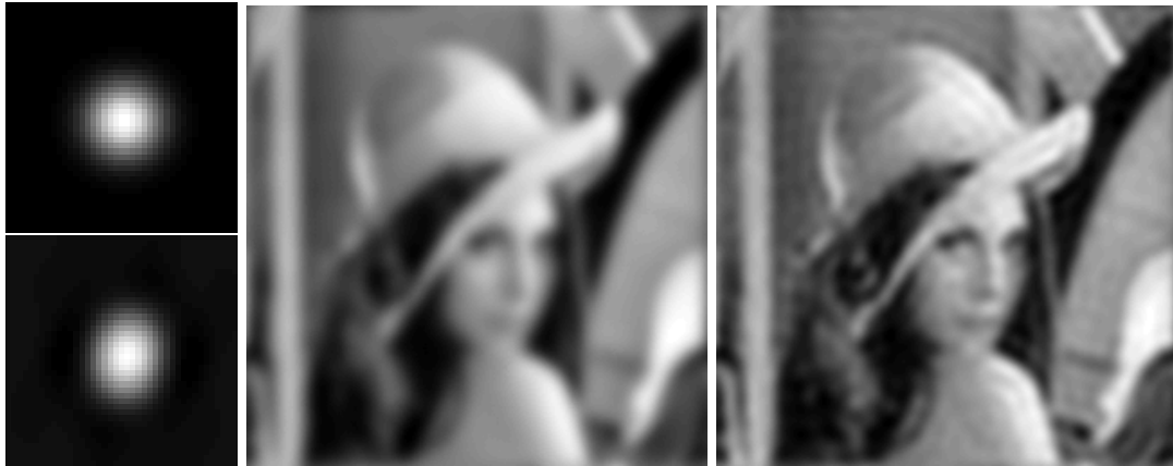
Figure 2: Gaussian PSF with large support. Images (left to right) of the true PSF that was used to generate the degraded image (top), the estimated PSF (bottom), the observed image and the estimated image.
