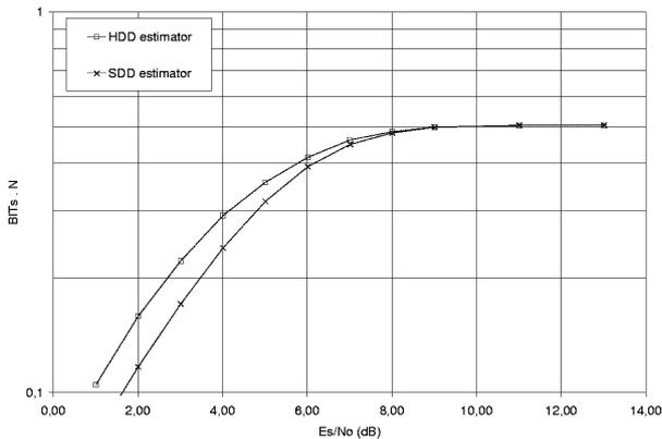
Figure 5: Equivalent noise bandwidths for the SDD and HDD estimators (obtained by simulation).
