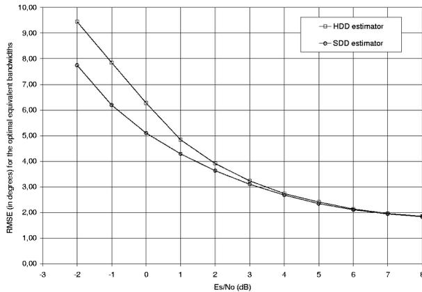
Figure 9: RMSE in presence of phase noise, with the HDD and SDD estimators and for the optimal estimation block sizes (QPSK modulation).
