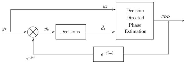
Figure 1: DD phase estimation with data pre-correction.
