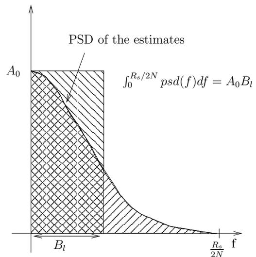
Figure 4: Definition of the equivalent noise bandwidth.
