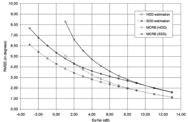
Figure 6: RMSEs and MCRBs for HDD and SDD algorithms (Constant phase error,  $N=32$ , QPSK modulation).
