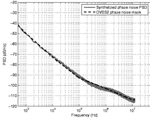
Figure 8: PSD of the synthesized phase noise and target mask
