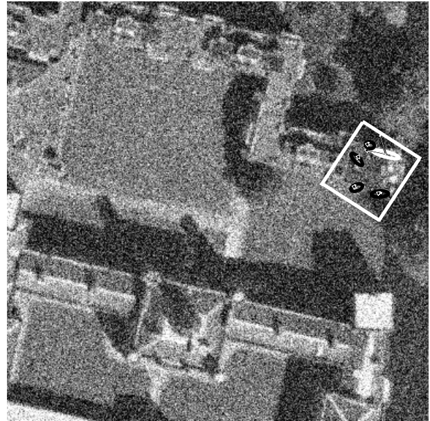
Figure 6: An example match of the target at 17.5% Gaussian noise, rotated 45^\circ . We display the correct match along with the associated candidates for the 15^\circ clusters from Figure 3, including the primary cluster.
