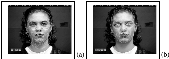
Figure 1: An example of mesh model fitting on a face image exploiting deformations.
