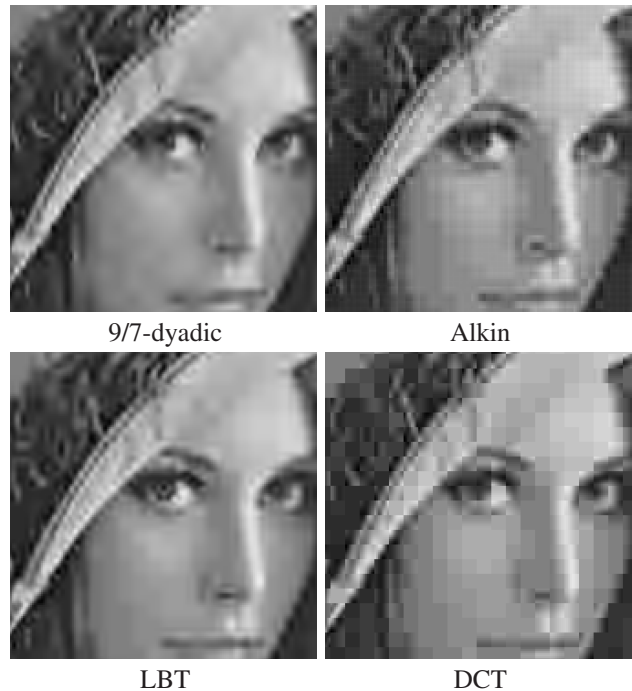
Figure 5: Zooms on reconstructed Lena images with the dyadic 9/7 transform and several 8-band transforms at 0.1 bpp with full reconstruction ( P = Q = 8 ).
