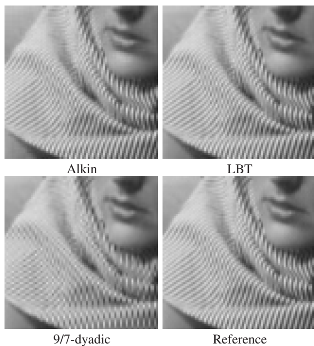
Figure 7: Zooms on reconstructed Barbara images reduced by a factor 8/6 with several 8-band transforms at 1.0 bpp with P = Q = 6 .
