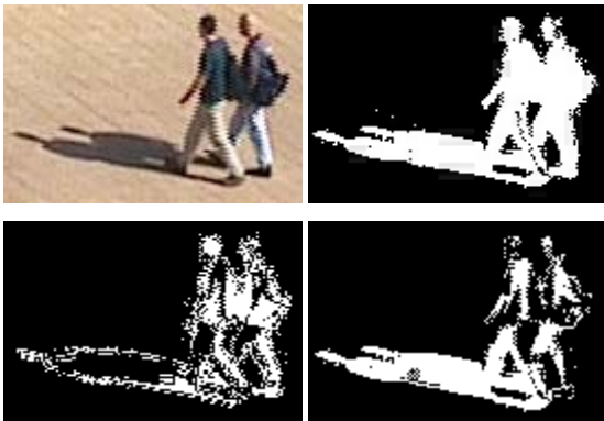
Figure 2 – Results of colour based shadow detection: upper left-input image, upper right-motion-detection mask, lower left-foreground mask determined by using colour features [5] and lower right-“worse-case” shadow mask ( \alpha=0.4 , \beta=0.8 ) used for input to classification method. (The binary masks are without morphological post-processing.)
