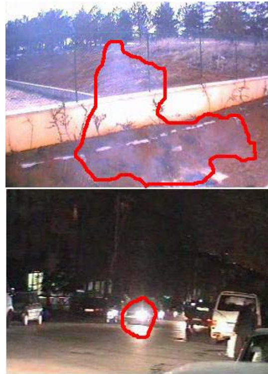
Fig. 4. Two moving objects in video: smoke image (top), and a vehicle (bottom). The object boundaries are determined by the background subtraction algorithm.
