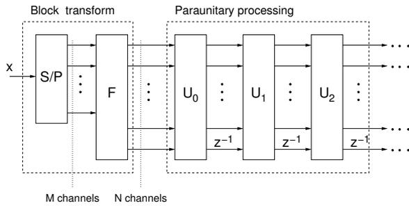
Figure 1: Lattice implementation of an oversampled filter bank satisfying equation (3).
