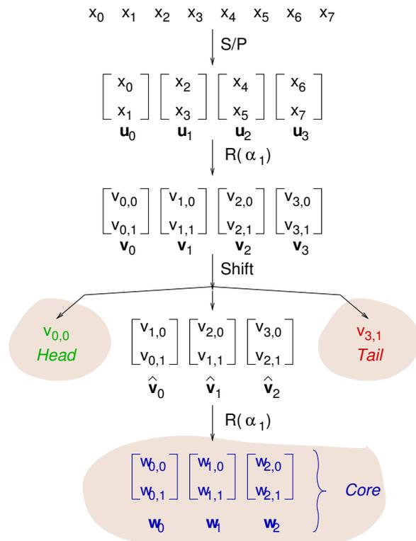
Figure 3: Example of the data generated by the scheme of Fig. 2a for an input signal of length  $2K = 8$ .
