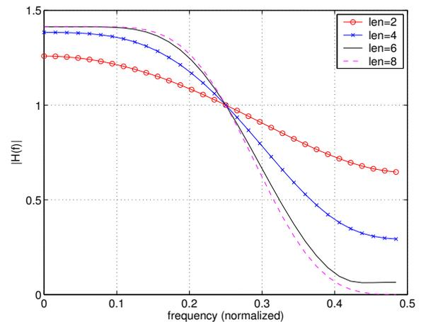
Figure 7: Frequency responses of the intermediate filters corresponding to an 8-taps Daubechies filter.
