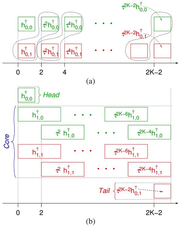
Figure 4: (a) Vectors corresponding to the output of the first rotation stage in Fig. 2a. (b) Vectors corresponding to the output of whole lattice structure in Fig. 2a. The topmost and bottommost blocks represent vectors inherited by the first stage and correspond to the *head* and *tail* part. The other blocks represent the translated version of the impulse responses of the original filter bank and correspond to the *core* part.
