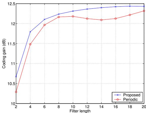
Figure 6: Comparison between the coding gains obtained by processing a finite length signal by using periodic extension and the proposed approach.
