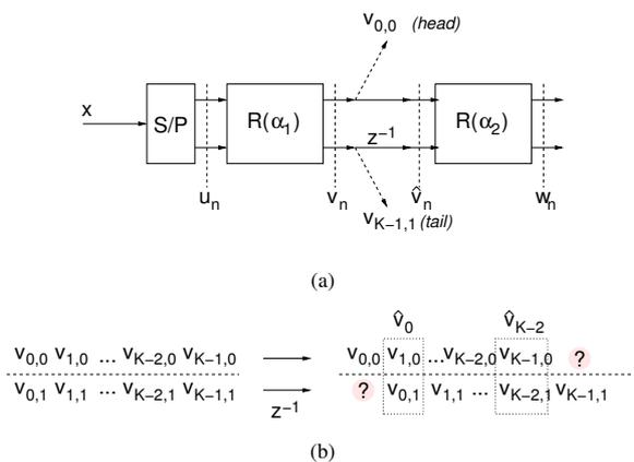
Figure 2: (a) Example of lattice implementation of an orthogonal two channel filter bank adapted to a finite support. (b) Effect of the shift stage.
