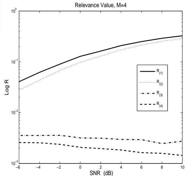
**Fig. 1.** Relevance value. Upper bound on the number of signals  $M = 4$ . The true DOA parameter  $\theta_0 = [28^\circ \ 36^\circ]$ , SNR =  $[-6 : 2 : 10]$  dB.
