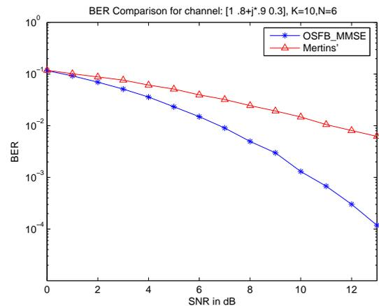
Figure 2: SNR\_BER comparison between our proposed OSFB\_MMSE design and Mertins' for channel=[1 .8+j\*.9 .3] with PLC noise,  $K=10, N=6$ .
