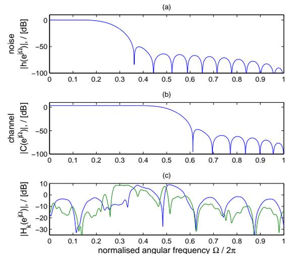
Figure 5: Magnitude responses of (a) lowpass noise (b) lowpass channel (c)  $N$  selected subband filters of the precoder for our OSFB design.  $K = 8, N = 2$  filters.
