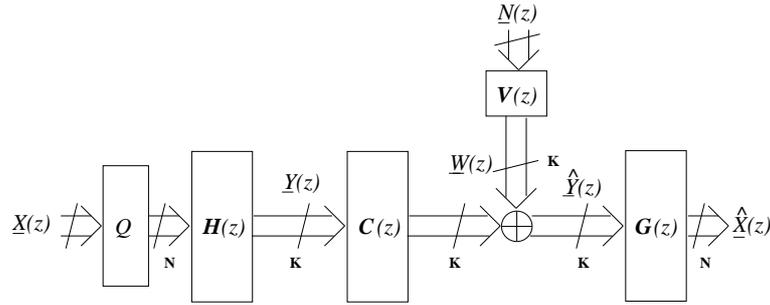
Figure 1: General model of the proposed OSFBs channel coding system.
