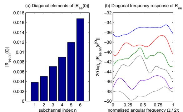
Figure 3: (a) Main diagonal elements of the system estimation error  $\mathbf{R}_{ee}(z)$ . (b) Frequency response of each subchannel estimation error  $\mathbf{R}_{ee}(z)$ .
