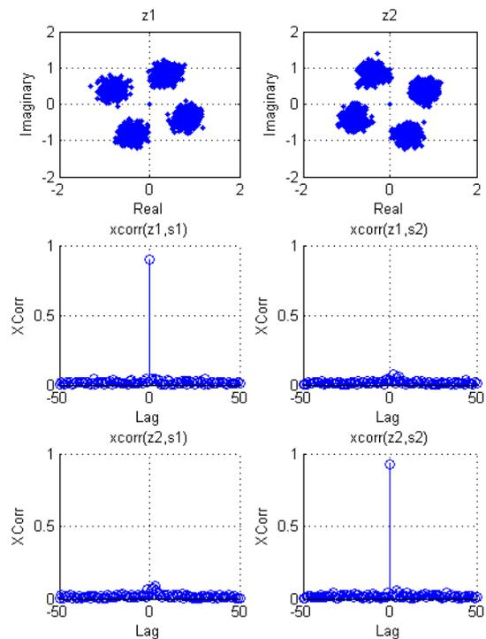
Figure 3: Equalizer outputs and cross correlation with transmitted sequences.
