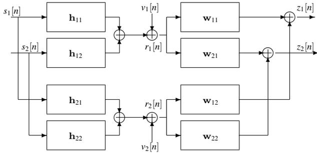
Figure 2: Channels and equalizers for a 2-by-2 MIMO system.
