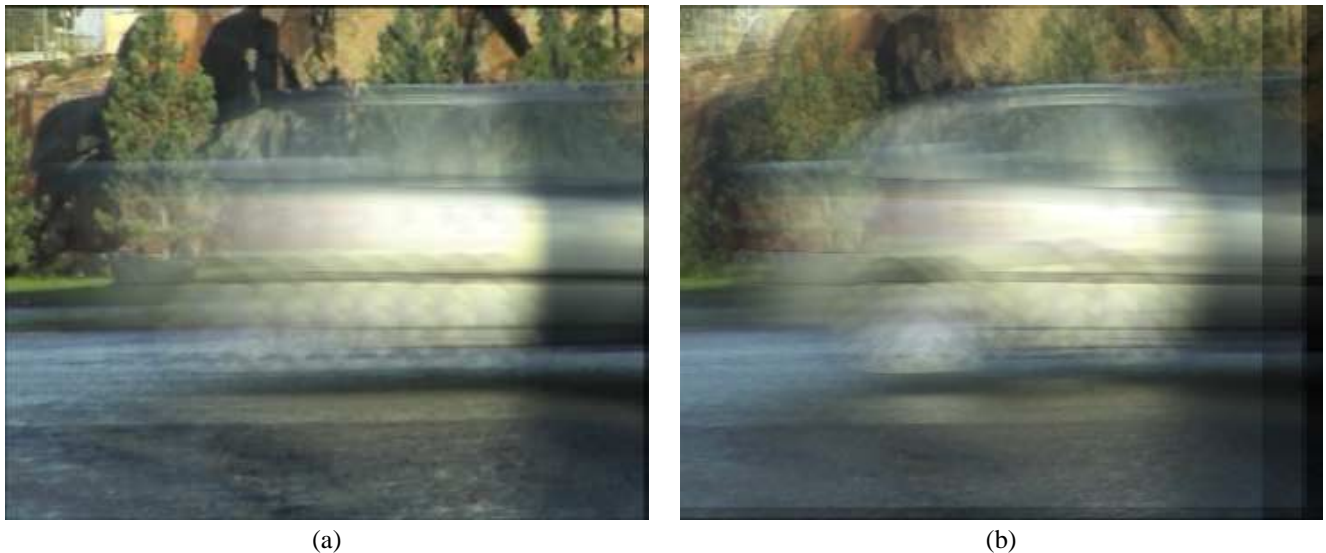
Figure 4: Several overlapped video frames after stabilization: (a) when using our method, (b) when using another method proposed in the literature. Note that the proposed approach is not disturbed by the moving object, being able to stabilize with respect to the static background that is sharp in the overlapped picture.
