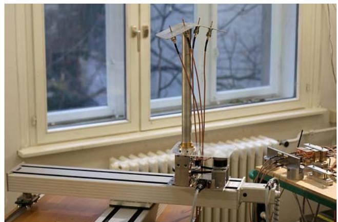
Figure 2: Receive antennas (moveable and rotateable) placed indoors.
