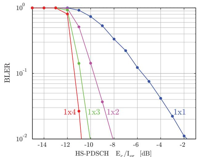
Figure 5: Block error ratios measured for a 1x1, a 1x2, a 1x3, and a 1x4 system
