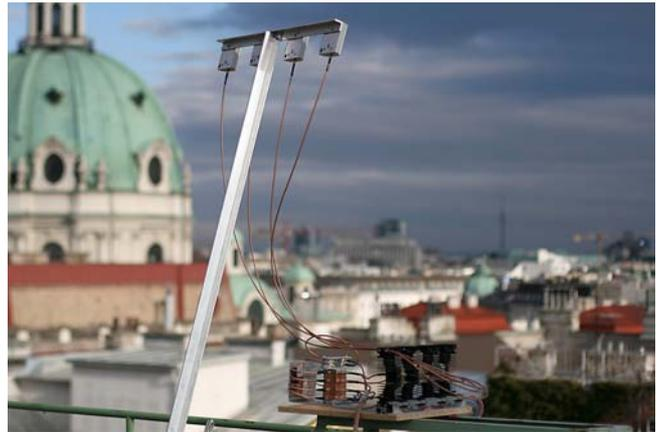
Figure 1: Transmit amplifiers and antennas placed on the roof.
