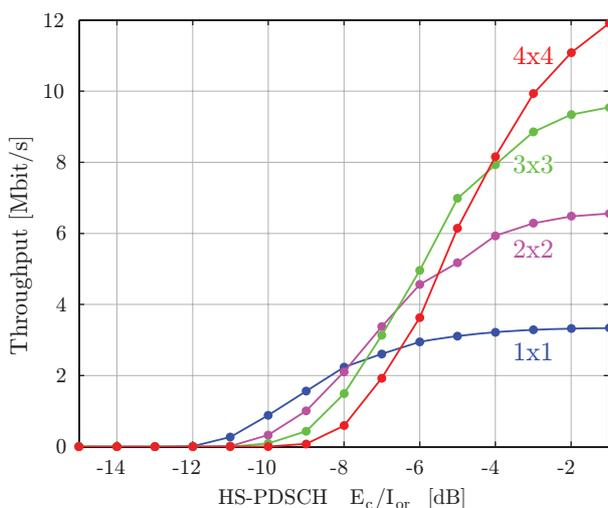
Figure 4: Measured throughputs averaged over channels for a 1x1, a 2x2, a 3x3, and a 4x4 system
