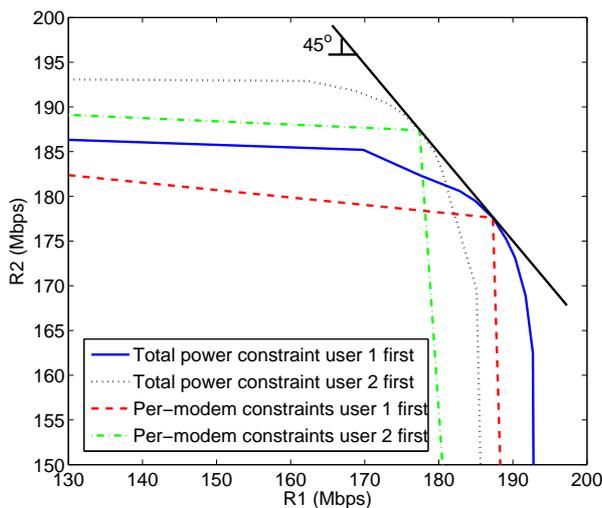
Figure 3: Rate region of BC-OSB in a complex gaussian channels
