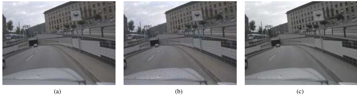
Figure 7: Comparison of the reconstructed HDR frames: (a) the original frame, (b) the Mantiuk et al. 's algorithm [7] (bpp=0.43, HDR VDP 75%=33.31%), (c) the proposed algorithm (bpp=0.26, HDR VDP 75%=23.32%). The images were tone-mapped to be printed.
