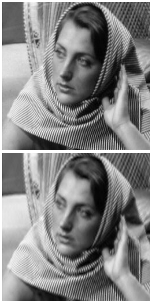
Figure 7: Top ) Zoom of Barbara image. Bottom ) Zoom of the decoded Barbara image using WANUS at bpp = 0.17 and PSNR = 27.41 db.
