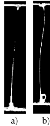
Figure 8: Segmentation results: a) Dropper, b) Dropper with electrical connection
