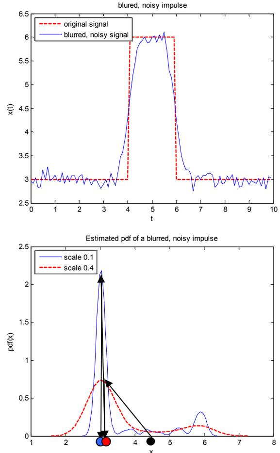
Figure 2 – Multiscale mode finding on 1D edge data. Up: noisy impulse. Down: Large scale pdf mode (red dot) is found first, then lower scale mode (blue dot) is precisely reached. Spurious modes around starting point (black dot) avoided.
