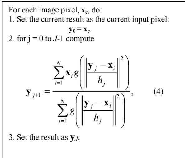
Figure 1 – Multiscale mode filter algorithm
