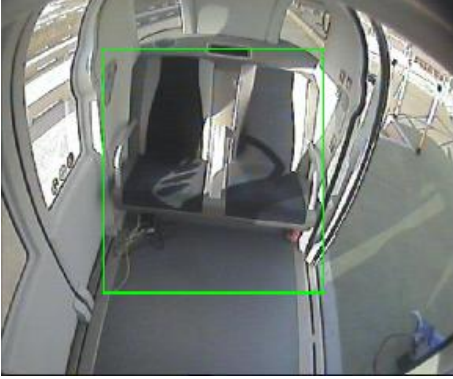
Figure 1: Interior of PRT vehicle with marked area of interest. The shadows caused by strong sunlight can be easily seen.
