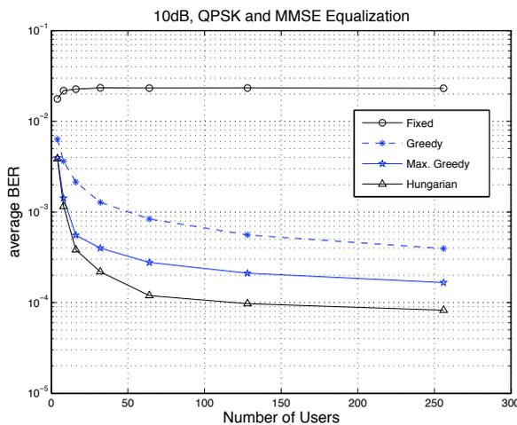
Figure 4: Effect of increasing users for different SA schemes with  $SNR = 10dB$
