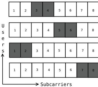
Figure 2: Localized SC-FDMA with  $N = 8$  subcarriers,  $U = 4$  users and  $M = 2$
