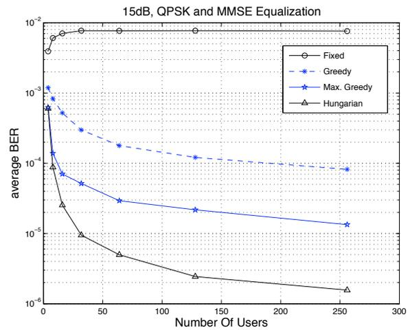
Figure 5: Effects of increasing users for different SA schemes with  $SNR = 15dB$
