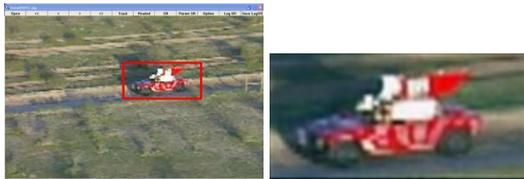
Figure 4: Selected object in the scene (left), and color SR reconstruction (right) with default settings proposed in section 4.3.3 and 20 images.
