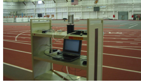
(b) The reference node equipped with directional antenna.
