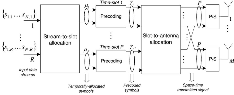
Figure 1: Proposed space-time spreading-multiplexing model as a cascade of 3 blocks: i) stream-to-slot allocation, ii) precoding, and iii) slot-to-antenna allocation.
