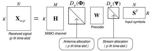
Figure 2: Visualization of the PARATUCK-2 decomposition of the  $p$ -th slice of the received signal tensor.
