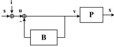
Figure 2: Equivalent linear model for the transmitter.
