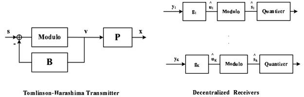
Figure 1: BC with Tomlinson-Harashima precoding.
