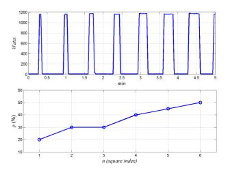
Figure 1- Example of a convector electric load ( $T_{00}$ =40s, A=1150 W)
