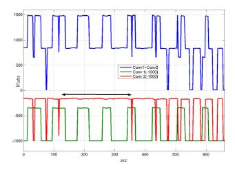
Figure 3- Electric load of two convectors operating simultaneously ( $T_{00}$ =80s for one convector Conv1 and  $T_{00}$ =40s for the other one: Conv2)
