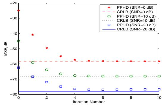
Fig. 2. Mean squared frequency errors versus iteration number  $k$ .
