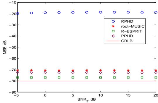
Fig. 4. Mean Squared frequency errors versus  $\text{SNR}_3$  for  $w_2$ .
