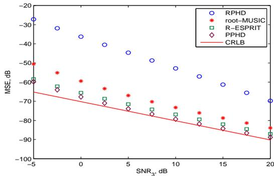
Fig. 5. Mean Squared frequency errors versus  $\text{SNR}_3$  for  $w_3$ .
