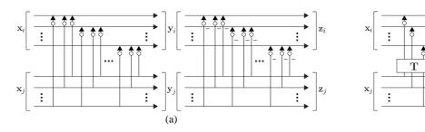
Figure 5: Block lifting structure: (a)before merging, (b)after merging rounding operations. (White circles: rounding operations.)
