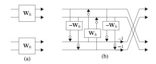
Figure 7: A block parallel system of PRFB: (a)basic structure, (b)parallel lifting structure. (White circles: rounding operations.)
