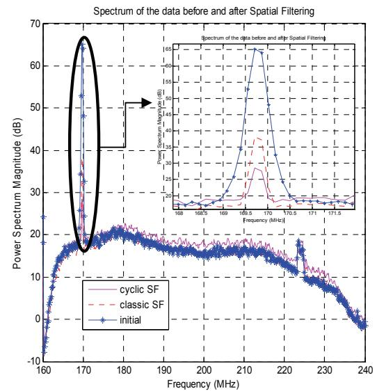
Figure 5 – Spectrum of one antenna output after applying cyclic and classic spatial filtering (M=8, L=65536).
