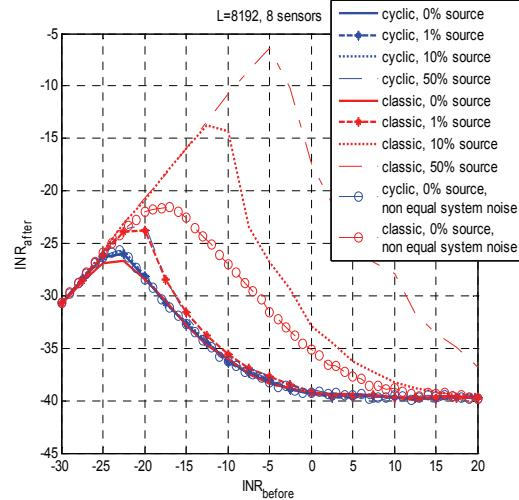
Figure 2 - Simulation results of the INR before and after applying spatial filtering, for 8192 samples and 8 antennas. The first 8 curves satisfy the “noise equal powers” assumption. For the last 2 curves, the noise powers fluctuate within 20% between antennas.
