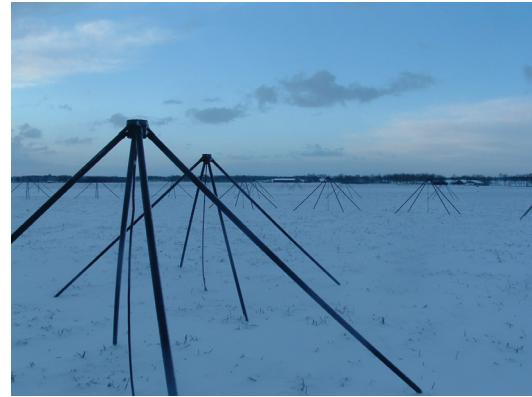
Figure 1: antennas of a low frequency radio telescope (LOFAR) station. The signals are combined by phased array beamforming and correlated with other LOFAR station signals. Sky images are produced by inverse Fourier transforming the correlation products.
