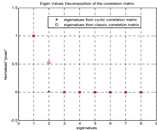
Figure 4 – The eigenvalue decomposition of the classic and the cyclic correlation matrix estimated from real data acquired with the LOFAR telescope. A strong transmitter is present in the dataset (see figure5). M=8 antennas have been used and the correlation matrices have been estimated over L=65536 samples.
