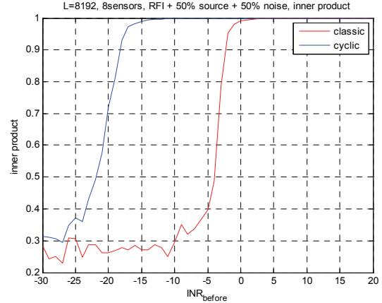
Figure 3 - Simulation results of the inner product between the true RFI spatial signature and the estimated one, for 8192 samples and 8 antennas. This inner product is equal to 1 if the spatial signature is accurate.
