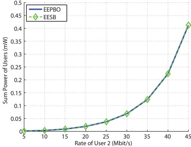
Figure 2: Sum-power transmitted for EEPBO and EESB when  $R_1 = 25$  Mbit/s and  $R_2$  varies between 5 and 45 Mbit/s.
