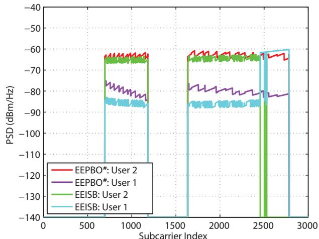
Figure 7: PSD's for EEPBO<sup>#</sup> and EEISB, which uses integer bit-loading, when  $R_1$  and  $R_2$  transmits 45 Mbit/s each.
