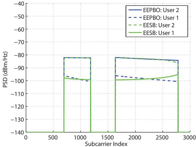
Figure 3: PSD's for EEPBO and EESB when  $R_1$  and  $R_2$  transmits 25 Mbit/s each.
