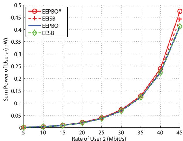
Figure 6: Sum-power transmitted for EEPBO<sup>#</sup> and EEISB when  $R_1 = 25$  Mbit/s and  $R_2$  varies between 5 and 45 Mbit/s.
