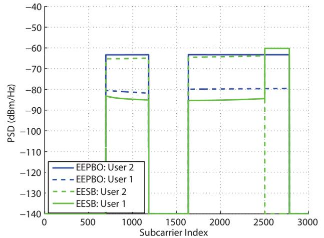
Figure 5: PSD's for EEPBO and EESB when  $R_1$  and  $R_2$  transmits 45 Mbit/s each.
