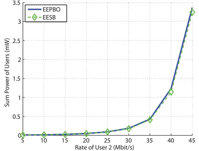
Figure 4: Sum-power transmitted for EEPBO and EESB when  $R_1 = 45$  Mbit/s and  $R_2$  varies between 5 and 45 Mbit/s.
