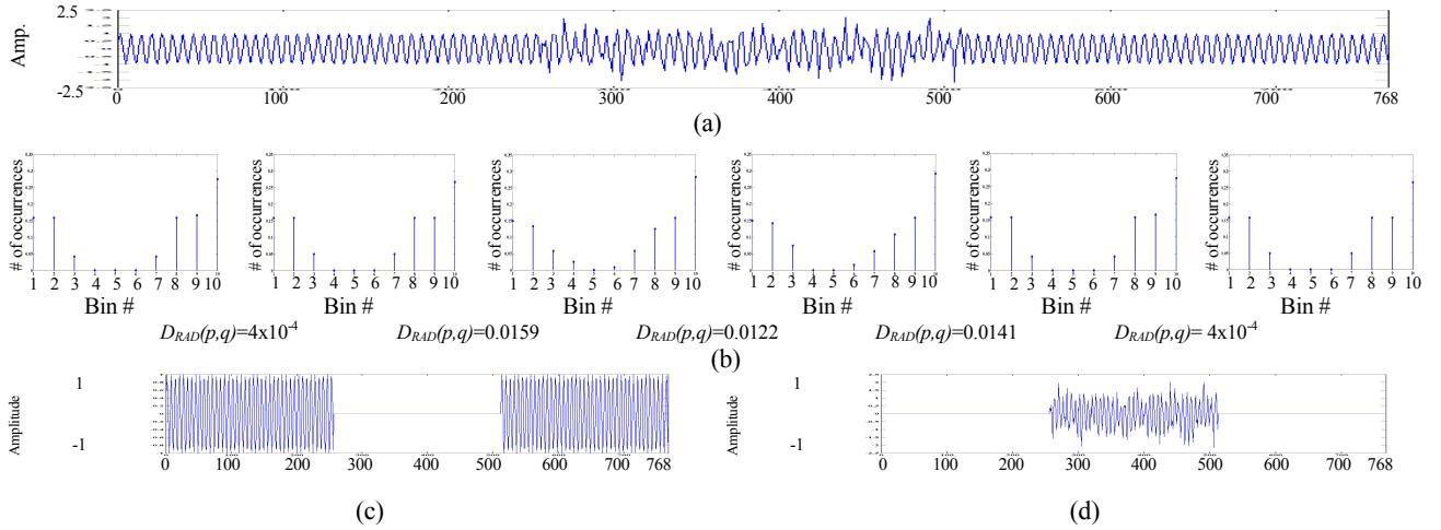
Figure 2 - Segmentation of a sinusoidal signal contaminated by AWGN (a) Original noisy signal (b)  $LBP_8^{r,u}$  histograms of the 6 segments formed and  $D_{RAD}(p,q)$  measure for adjacent histograms (c) Segmented sinusoidal components (d) Noise affected segment
