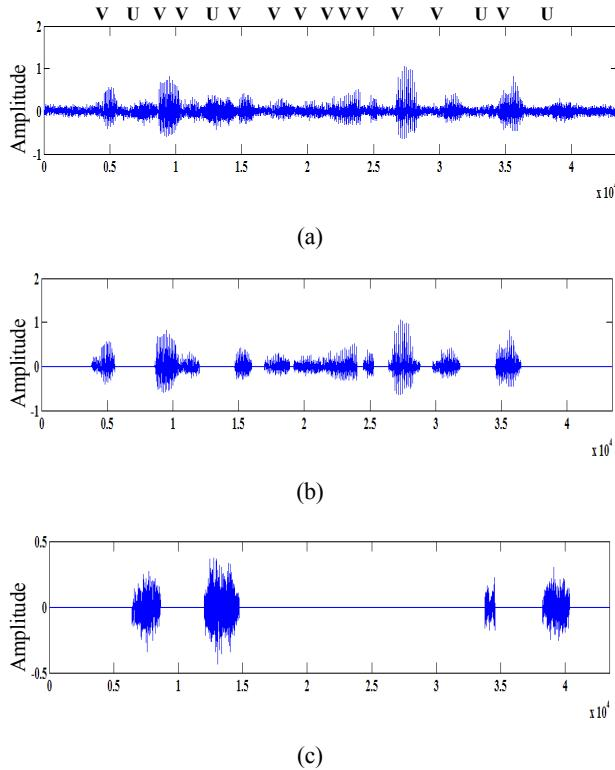
Figure 4 - VAD results for speech contaminated with F16 cockpit noise at 5 dB SNR (a) Noisy speech (b) Voiced speech components identified (c) Unvoiced speech components identified
