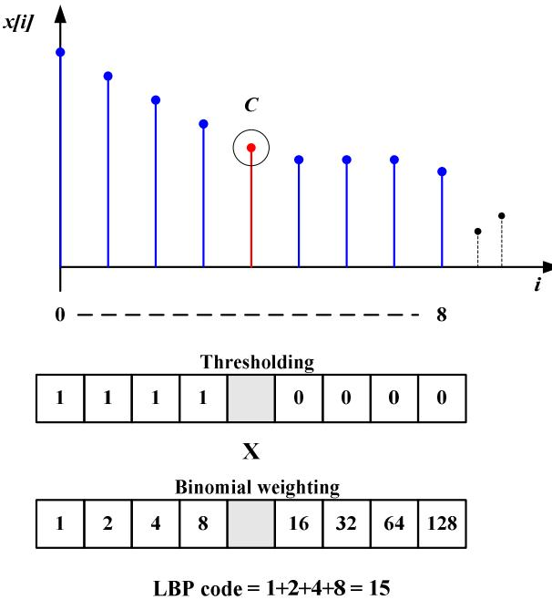
Figure 1 - Computation of 1-D local binary pattern (1-D LBP)
