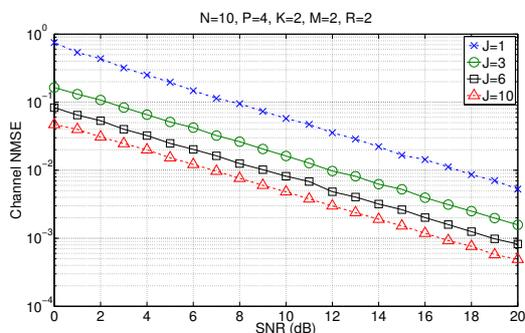
Figure 1: Influence of  $J$ : Channel NMSE versus SNR.
