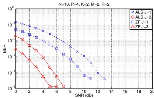
Figure 5: Comparison of TST-ALS and TST-ZF receivers.
