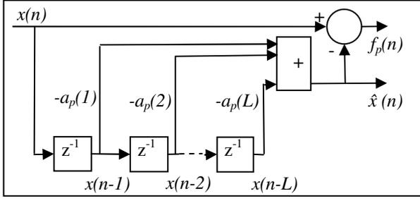
**Figure 1 Forward Linear Predictor**
