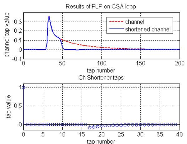
**Figure 7 Channel 3, DFLP and Effective Channel IRs**
