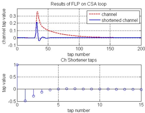
**Figure 4 Channel 3, FLP and Effective Channel IRs**
