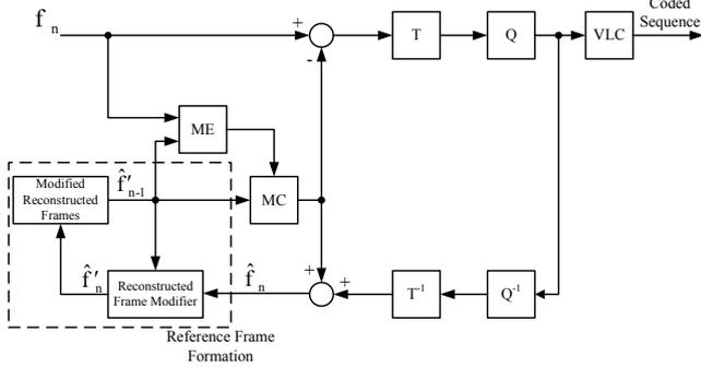
Figure 1: Block diagram of a video encoder with reference frame modification. (ME, MC, T and Q represent Motion Estimation, Motion Compensation, Transform and Quantization respectively).
