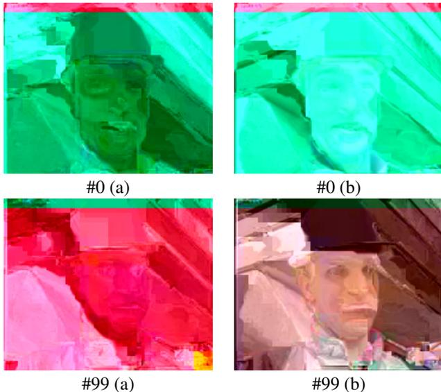
Figure 10: a) Images of *foreman* in QCIF compressed with QP=12 while using SE-CAVLC [6], b) Corresponding images while applying RSE.
