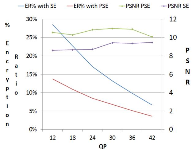
Figure 9: PSNR and ER of *foreman* while applying SE [6] and RSE for a wide range of QP.
