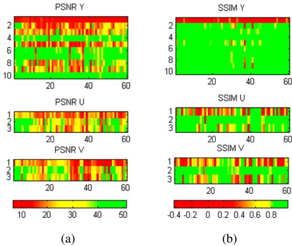
Figure 7: PSNR and SSIM [8] of "mobile" in QCIF with QP 12 for the 60 first frames, only the 26th macro-block is encrypted.
