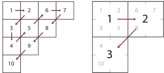
Figure 2: Zigzag scan of the ten closer macro-blocks of the single encrypted block for *luma*, and zigzag scan of the three closer macro-blocks of the single encrypted block for *chroma*
