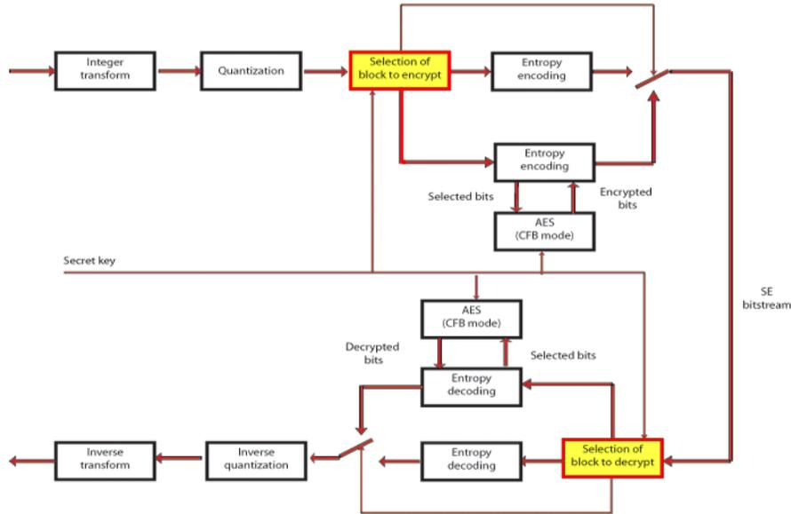
Figure 1: Block diagram of encryption and decryption process in RSE-CAVLC.
