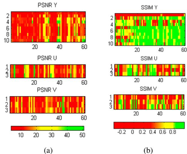
Figure 6: PSNR (a) and SSIM [8] (b) of "Mobile" in QCIF with QP 12 for the 60 first frames, only the first macro-block is encrypted.
