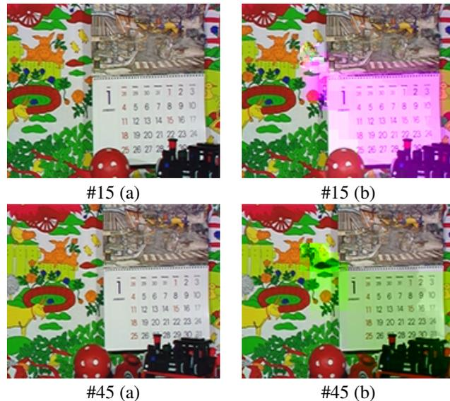
Figure 5: a) Original images of "mobile", b) Corresponding images where only the 26th block is encrypted with SE-CAVLC [6].
