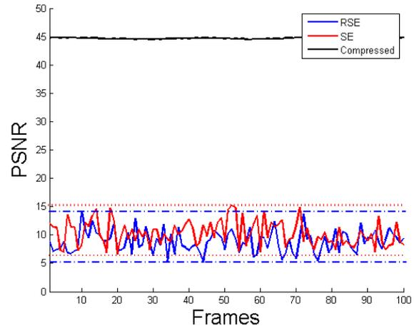
Figure 8: PSNR of *foreman* for 100 frames while using SE [6], RSE and a standard H.264/AVC compression with QP=18.
