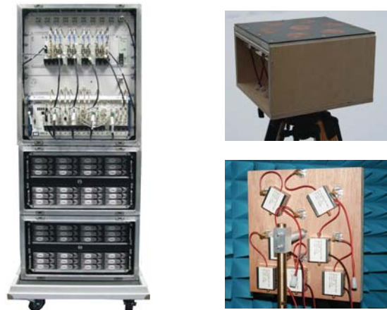
Figure 1: 8-channel recording system ECHSE (left) and 7-element GPS antenna IKARUS (right).
