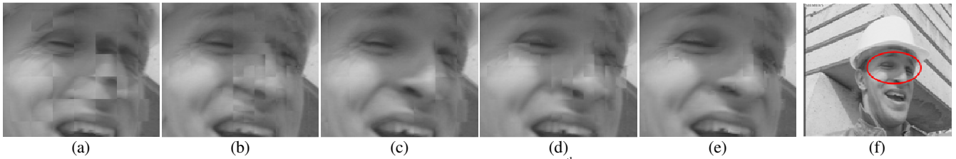
Figure 8 – Comparison of the original frame and the interpolated frames of the 14 th frame within Forman (CIF). (a) MCFI, (b) OBMC, (c) Thaipanich et al. , (d) Oh et al. , (e) proposed algorithm, and (f) original frame.
