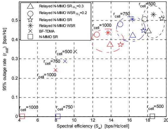
Figure 2 - Outage transmission rate ( $r_{out}$ ) vs. spectral efficiency ( $S_e$ ) for different transmission strategies and  $F=1$ , using and not using RS. Cell radiuses are 500 m (black), 750 m (red) and 1000 m (blue).
