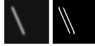
**Fig. 3.** Particle trajectory with 70 degree angle (left) and filter results for  $S_x^+$  and  $S_x^-$  overlaid in one image (right).
