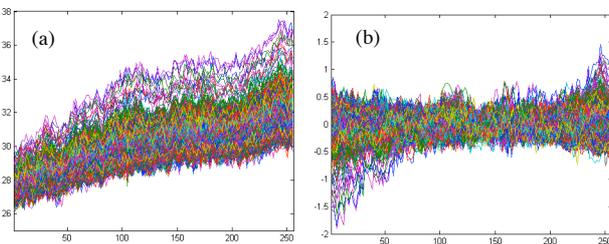
Figure 4: Several responses over time recorded by the IR camera (a); Signals after removing trend and noise (b), which can be interpreted as realizations of a stationary process.
