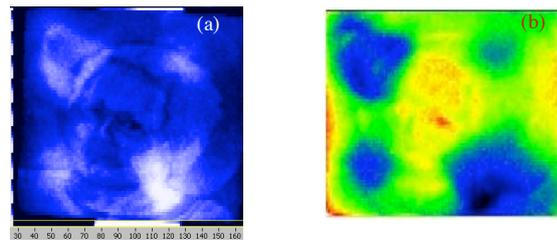
Figure 6: Defects estimation with other methods [15-17]: best contrasted image from an acquisition with a classical step heating excitation (a); results of a parametric analysis of the response to a PRBS excitation (b).
